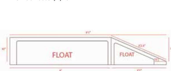
Figure 2: Side view of float structure for New York Aquarium Harbor Seal exhibit. Hubbert, J., 2022
